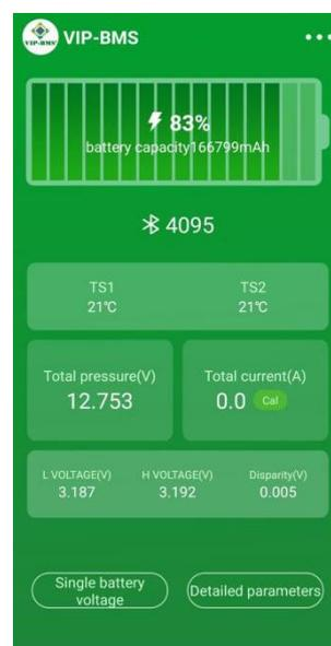
**\*\*Note: the battery MUST get a fully charge and discharge cycle then you can get an accurate battery capacity\*\***
